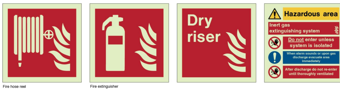
Figure 4: BS EN ISO 7010 fire fighting equipment sign(s) & fire safety notice(s).
